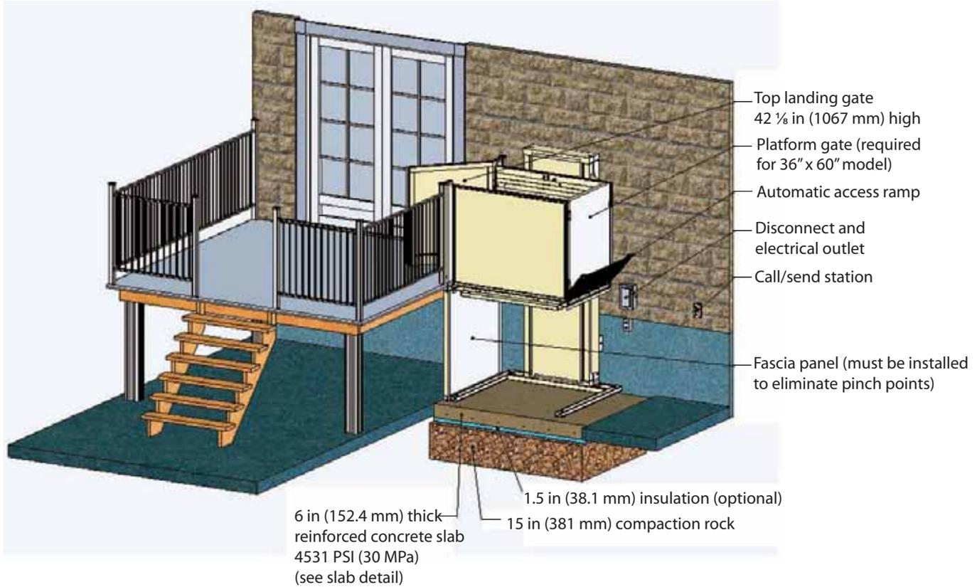
Outdoor applications need a strong and stable surface that will not move throughout the years. For this reason, it is essential, when the temperature can get below the freezing point, to insert an insulate sheet between the concrete slab and the compaction rock. Figure 6 illustrates the concrete slab detail for a typical outdoor application.
