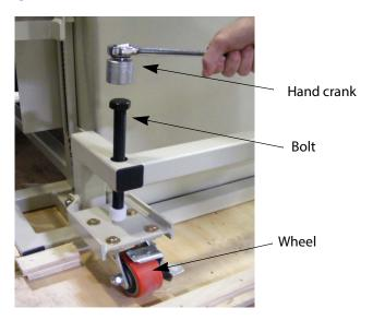
2 Roll lift into position at the landing level where it will be used. Using the handcrank, raise the wheels off the floor and ensure the plate above each wheel is activating the push button switch as shown below. Lock down the wheels as shown in the next figure.
